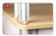
Screw the stand-off's down onto the stand-off locators until fully secure. Repeat this for the remaining stand-off's
